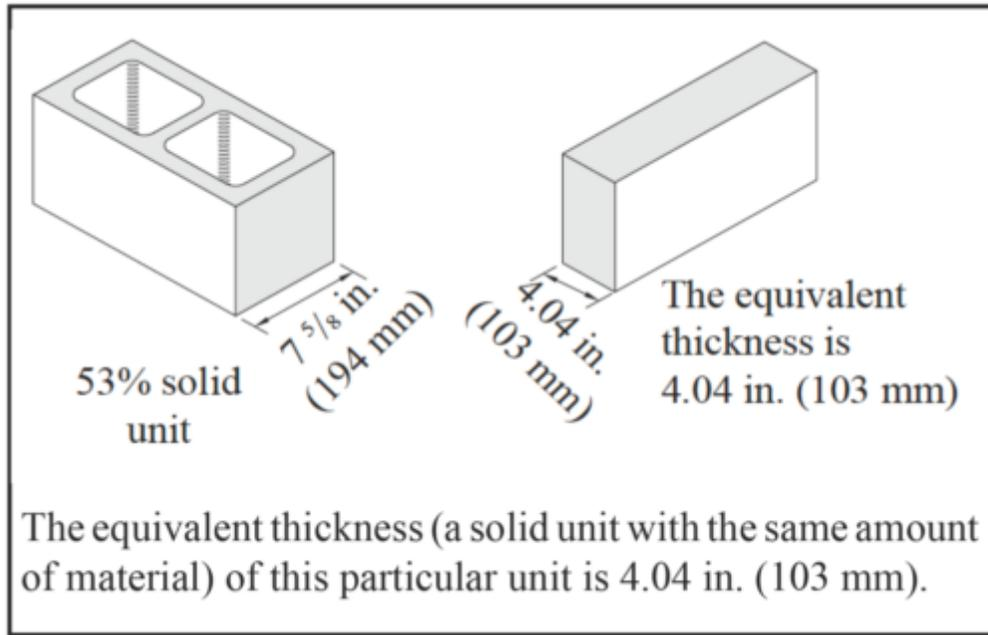
Figure 1—Equivalent Thickness
